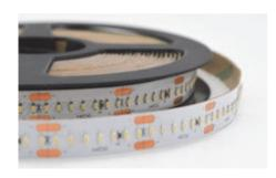
Input voltage 24V Power/m 19.2w/m CRI(Ra) >90 Beam angle 120° LEDs/m 280LEDs -25°C~+45°C Working temperture 50000h Working hour PCB Width 10mm
