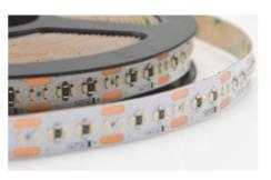
Input voltage 24V Power/m 20w/m CRI(Ra) >90 120° Beam angle LEDs/m 300LEDs Working temperture -25°C~+45°C 50000h Working hour PCB Width 10mm
