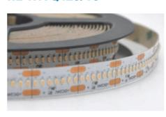
24V Input voltage Power/m 20w/m CRI(Ra) >90 Beam angle 120° LEDs/m 420LEDs -25°C~+45°C Working temperture 50000h Working hour PCB Width 10mm
