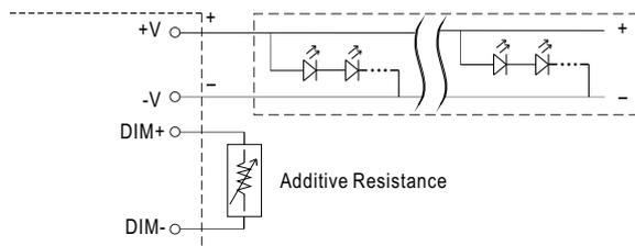
"DO NOT connect "DIM- to -V"
