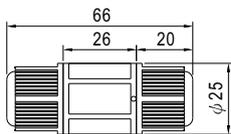
CJ04-1 suitable for 14AWG~16AWG
