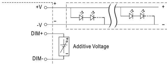
"DO NOT connect "DIM- to -V"
