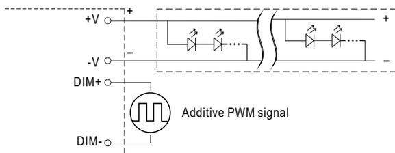
"DO NOT connect "DIM- to -V"
