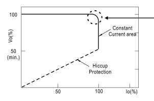
Typical output current normalized by rated current (%)
