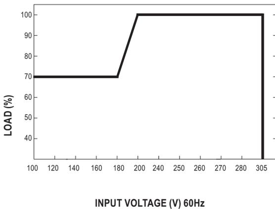
※ De-rating is needed under low input voltage.
