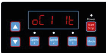
Diagram 4.25, Auto Recovery, error details OC1, error time 1
