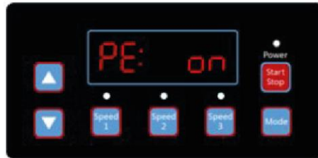
Diagram 4.23, Self-Priming Enable/Disable, default On
