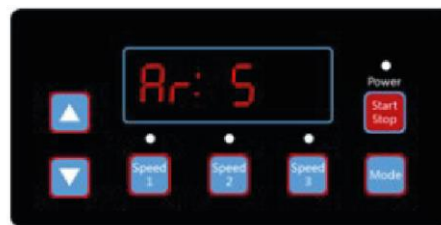
Diagram 4.26, Auto Recovery count down, 5 seconds remaining
