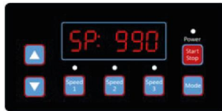
Diagram 4.11, 1000 RPM press “Down” once
