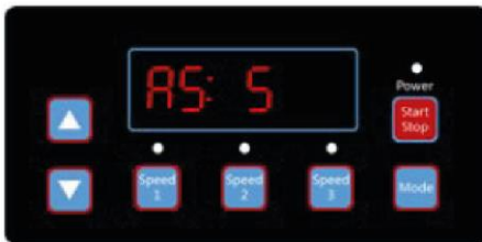
Diagram 4.27, Auto Start count down, 5 seconds remaining
