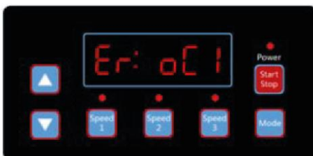
Diagram 4.28 Error, Error code OC1
