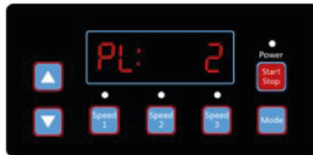
Diagram 4.21, Self-Priming Time, default 2 min
