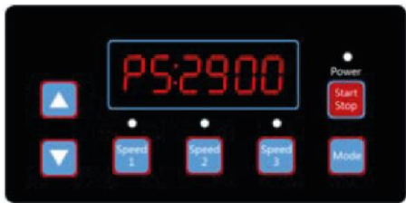
Diagram 4.22, Self-Priming Speed, default 2900 RPM
