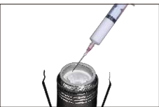
Use the Silicone with good stickiness and thermal effect for reach the purpose of radiating and prevent moisture.
