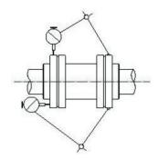
If non alignment is found, please use the adjustment system on the base to align the shaft.
