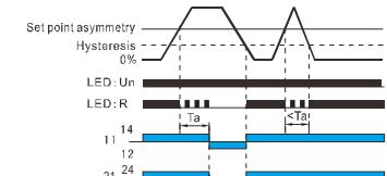
To:Overvoltage threshold tripping delay.
