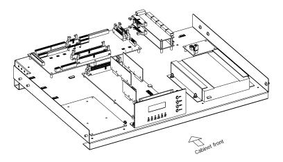
Figure 11 Structure of Monitoring Unit
