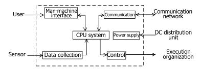
Figure 12 Principle of Monitoring Unit
