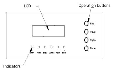
Figure 14 Front Panel of Monitoring Unit
