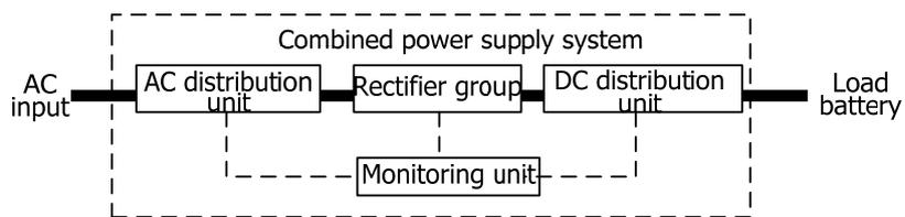
Figure 4 System Principle
