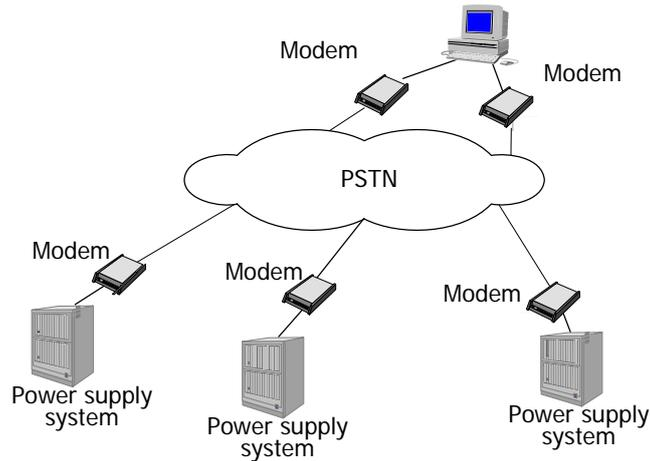
Figure 16 Monitoring in the Modem Mode
