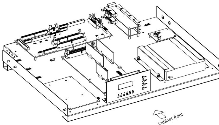
Figure 11 Structure of Monitoring Unit
