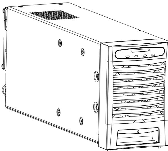
Figure 6 Appearance of ZXD2400(V4.0) Rectifier
