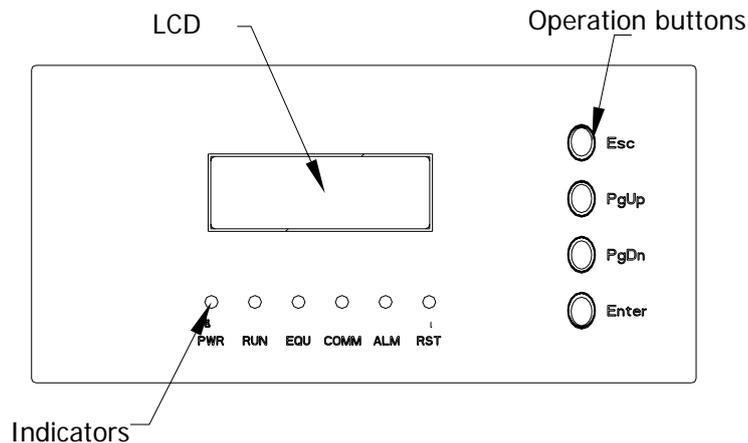
Figure 14 Front Panel of Monitoring Unit
