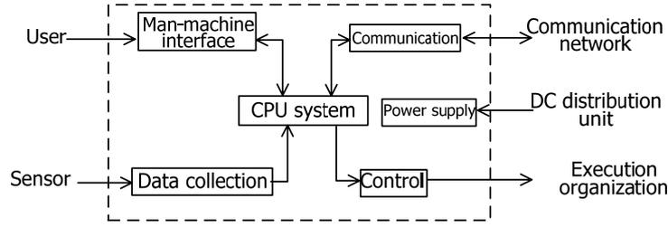
Figure 12 Principle of Monitoring Unit
