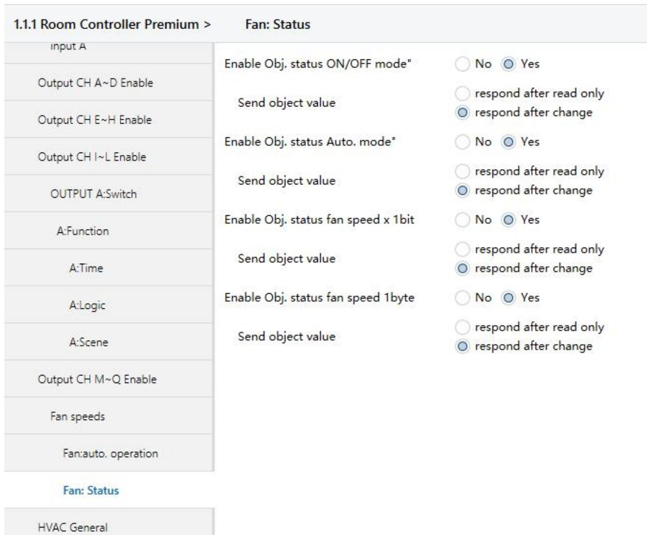
fig.5.37 Parameter Settings interface “Fan-multi level: Status”
