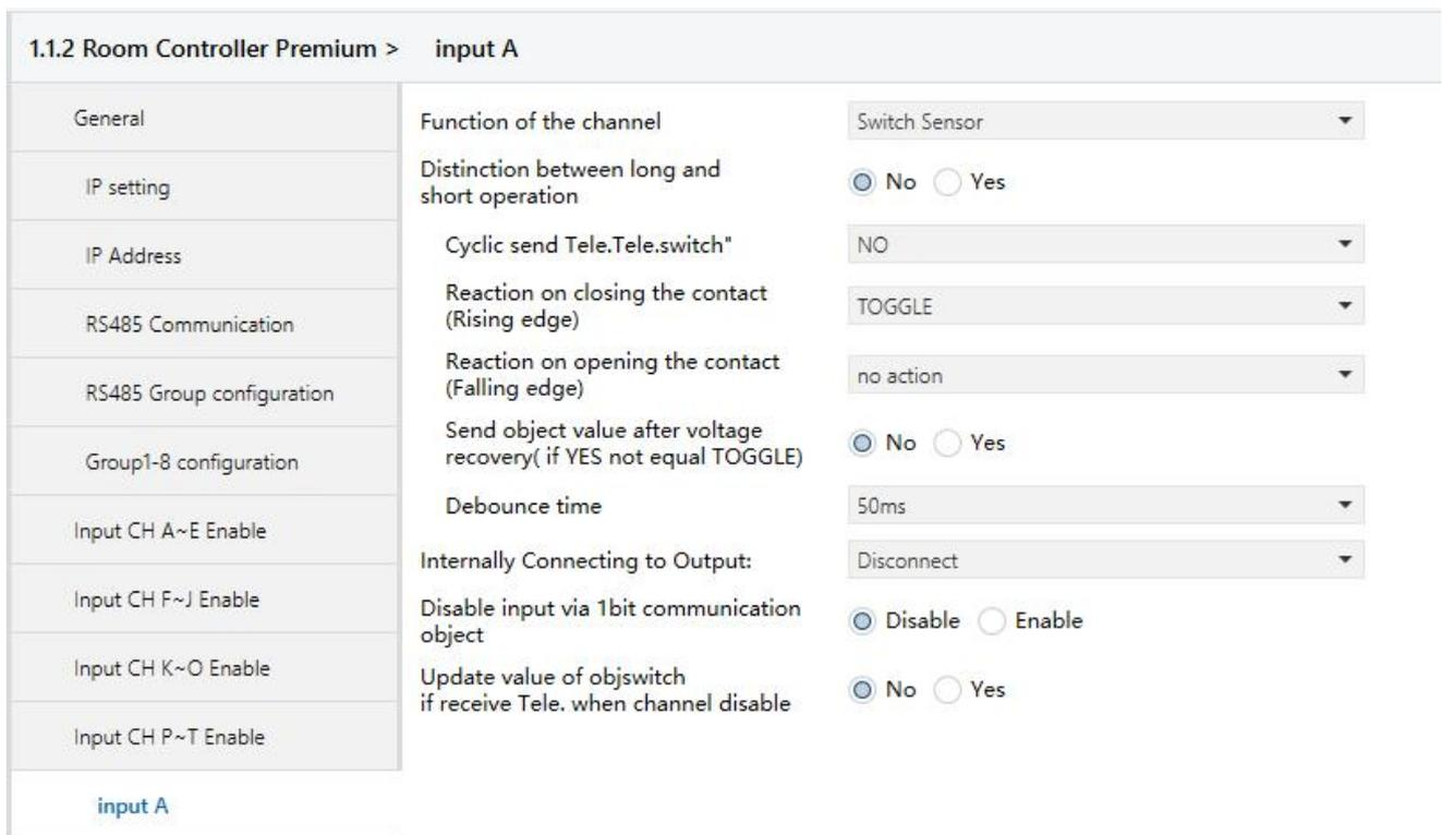
Fig.5.9 Parameter window "Switch X" (Distinction long/short operation)
