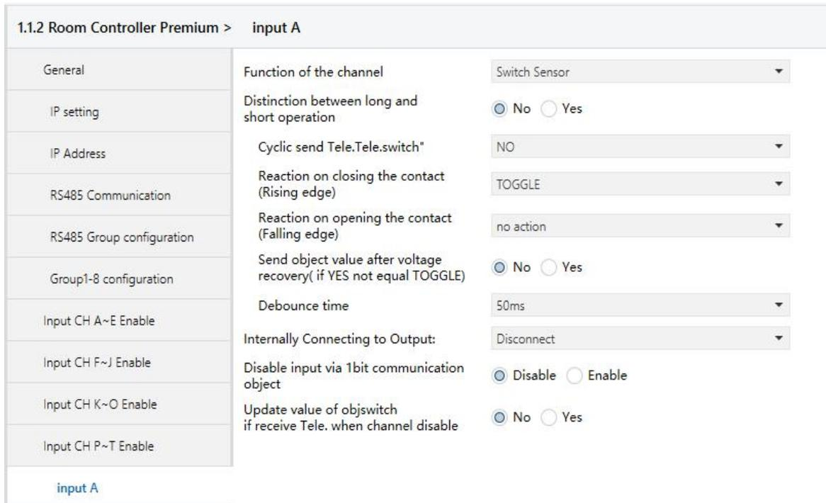
Fig. 5.8 Parameter window “Switch sensor” (No distinction long/short operation)
