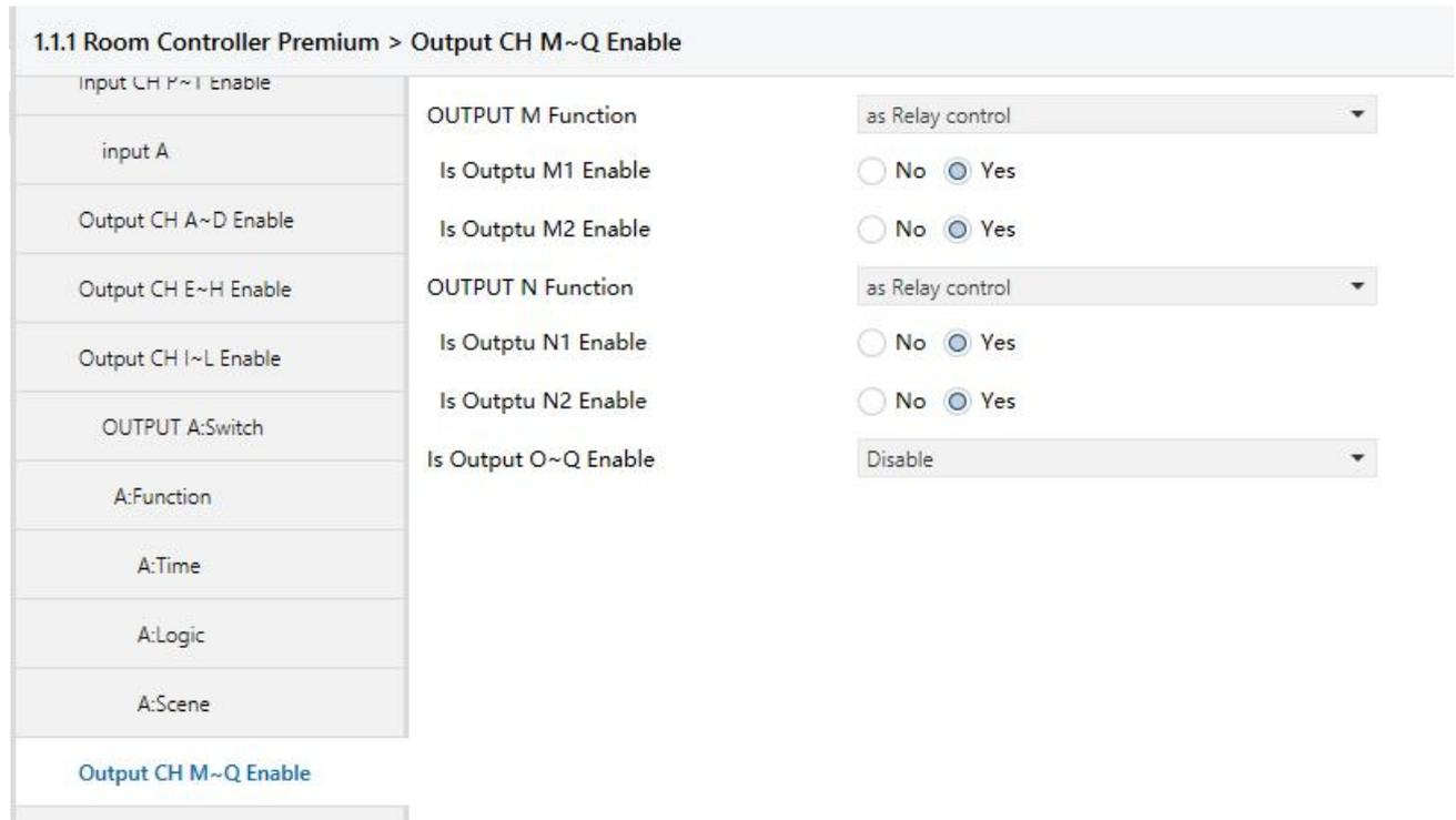
Fig.5.30Parameter window “Switch- outputs M1,M2,N1,N2”
