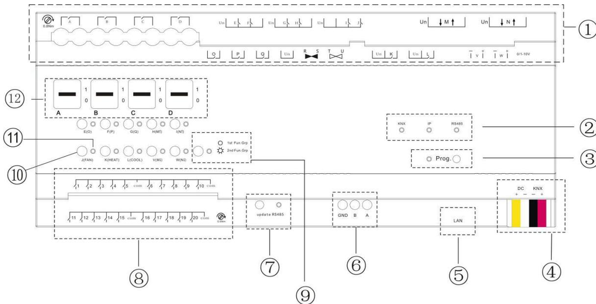
① Output terminals: A~L are switching outputs; V and W are dimming outputs; OPQ are fan speed outputs; R and S are for heating valve; T and U are for cooling valve; M and N are shutter outputs
