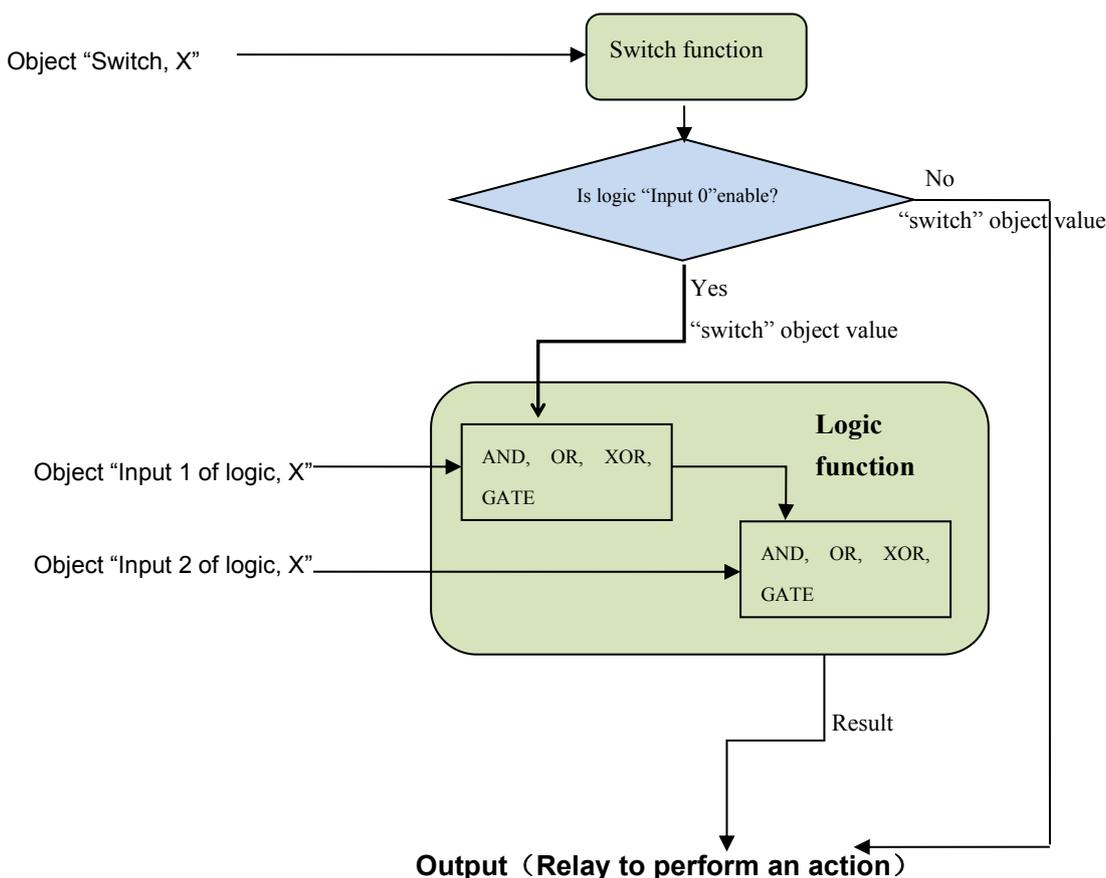
Fig. 5.15 switch and logical function diagram
