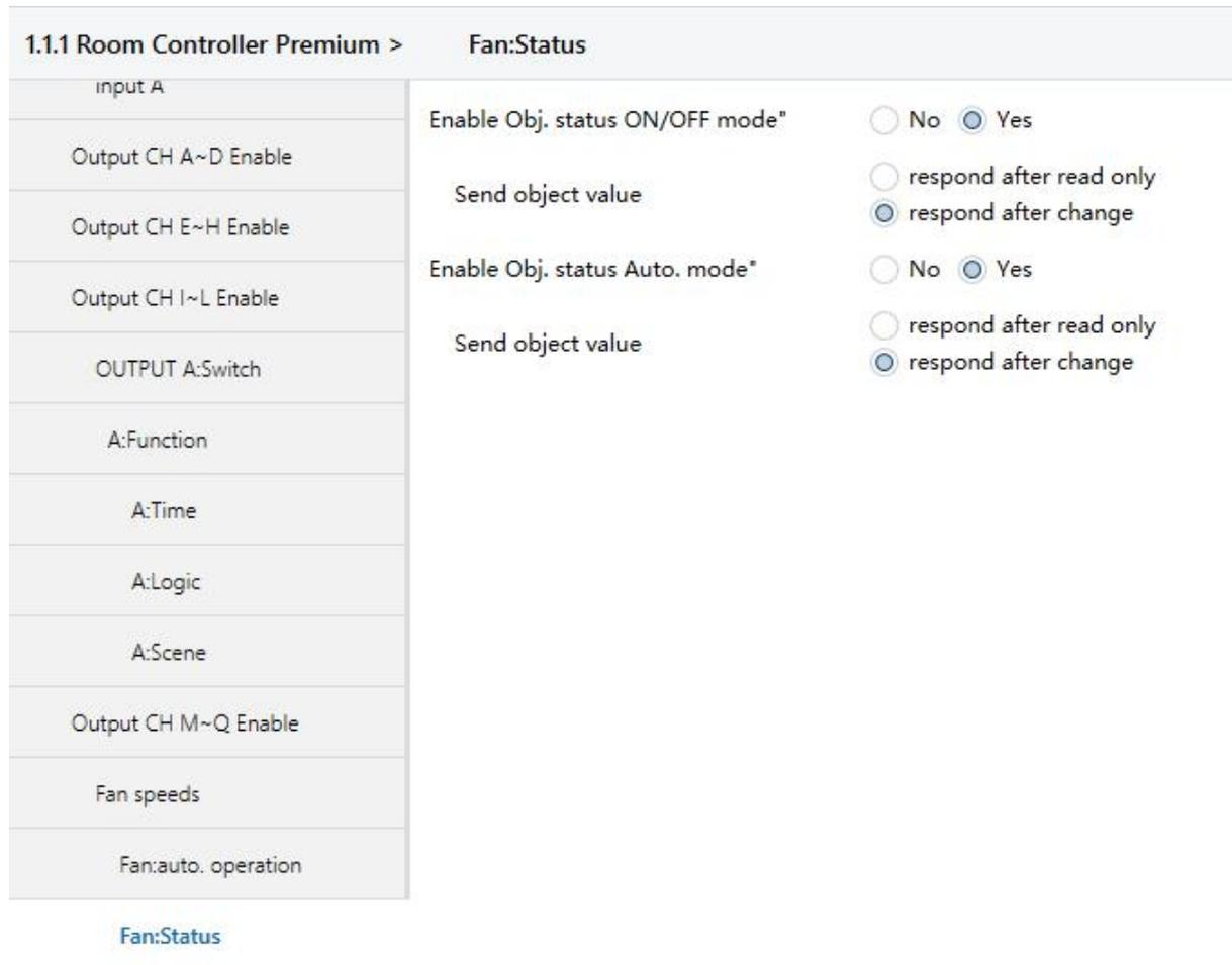
Fig.5.34 Parameter window “Fan-one level: Status”
