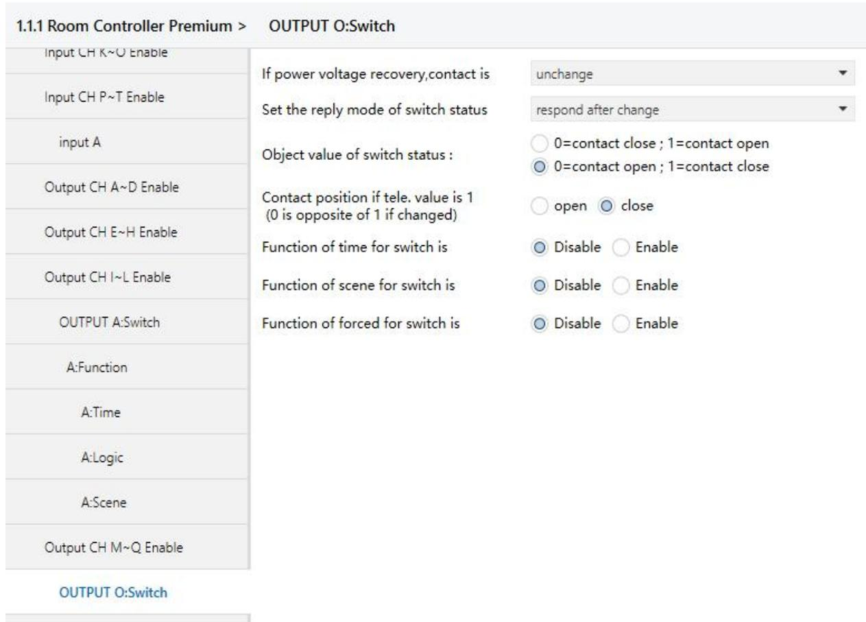
Fig. 5.38 Parameter setting interface of “Switch- outputs O,P,Q”
