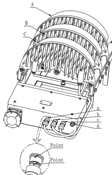
**Notice:** The white dots on male and female terminals are positioning point, can only be plugged in when they are matched. Tightly screw the nut on the aviation plug to avoid poor wire contact.
