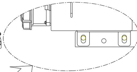
5. Using 4 sets of M12 bolt set unscrewed from step 2, tightly mount the set of step 3 onto the bracket through 4 mounting holes on the side.
