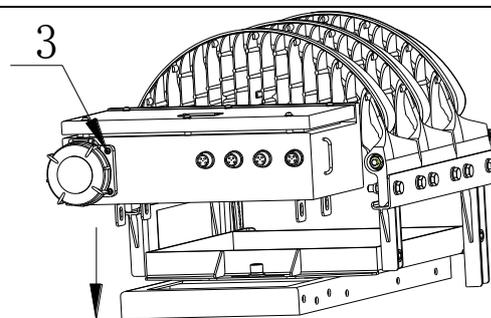
4. Make sure the mounting hole position of the junction box is the same as the light's bracket; use 4 sets of M10 bolt set unscrewed from step 2 to fix the junction box onto the light's bracket. Notice: During the whole assembly process, please make sure there is no collision between the light's wiring harness and the aviation plug.
