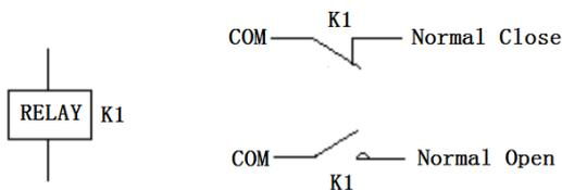
The lights are connected to the power supply and are working properly:Relay action, "common terminal" and "normal open terminal"close, as below:
