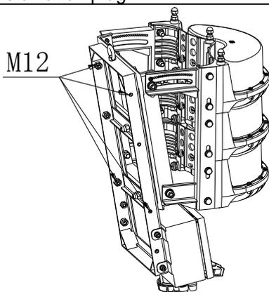
6. After fixing the light head, put the Gradienter (no. 11) on the top of the light case to make sure the light is fixed horizontally. If the light is not fixed horizontally, please adjust according to step 7 (below).
