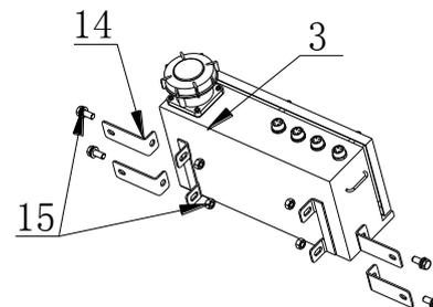
3. Please install the junction box vertically onto the light bracket, make sure the aviation plug facing outward.
