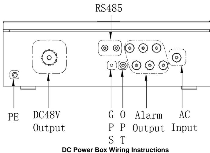
6. Power box internal wiring instruction (please refer to the wiring label inside the power box). Before connection, please make sure the air switch of input terminal is off:
