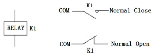
•If there is no power access, or failure are received "disconnect" signal, the alarm signal line connected to the "common" + "normally open".
