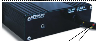
External connection cable and power cable
