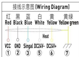
It is recommended to use RVVP/0.5mm/copper core/low temperature resistant shielding cable, maximum communication distance is 1000m.
