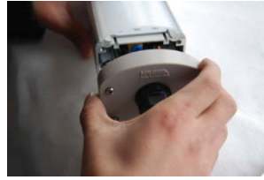
2. Pull out the cover and wire terminal revealed.
