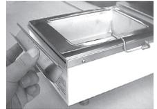
3. The level of the melted solder should be about 1cm below the top edge of the pot.
