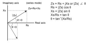
There are two types of reactance. One is inductive reactance  $X_{\rm L},$  and the other is capacitive reactance  $X_{\rm C}.$
