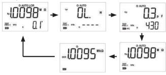
In the manual LCR mode, the meter automatically selects the series/ parallel mode depending on the total equivalent impedance measured similarly to the Auto LCR mode. (Refer to 4-7)
