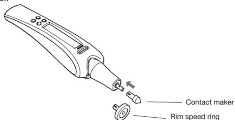
\* Select the rim speed ring when measuring the velocity of a belt conveyor or similar object (Travel distance per minute in m/min or travel distance per second in m/s).
