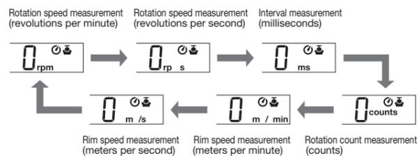
When the rim speed ring is attached, select either the [m/min] or [m/s] mode.
