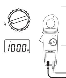
needed. Read the result from the LCD display.
