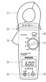
① Current Sensing Clamp ② Barrier (3) Clamp opening handle (4)LCD display  $(\overline{\mathbf{5}})$ COM input terminal (6) Positive input terminal ⑦ Function selector Data hold button (8)
