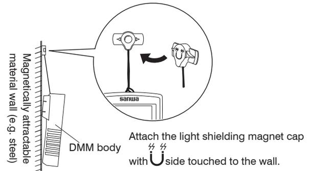
Attach the light shielding magnet cap with U side touched to the wall.
