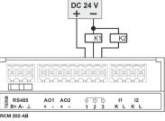
Fig. 5: Connection of two relays to the digital outputs
