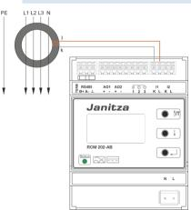
Fig. 3: Simplified presentation of residual current measurement
