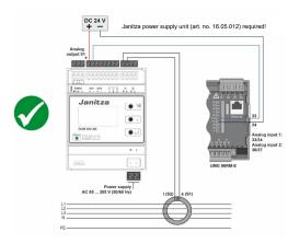
Fig. 7b: Connection to the analogue outputs of a UMG 96RM-E
