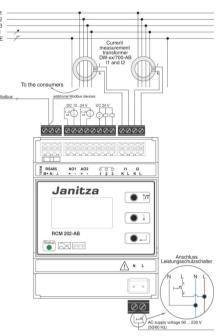
Fig. 4: Circuit diagram of the RCM 202-AB
