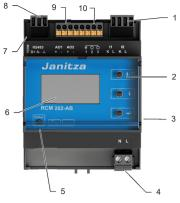
Fig. 1: RCM 202-AB device view
