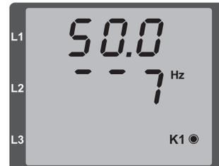
Example 1: Fig. Display of the mains frequency (50.0 Hz) and the phase sequence.
