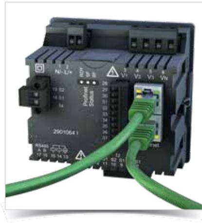
Fig.: UMG 96RM-PN with Profinet interface
