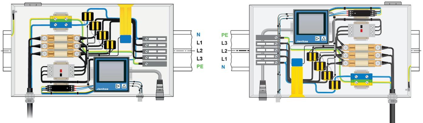
A choice of two possible cable outlets allows easy adaptation to the installation situation. In the version with a display, the measurement device can be rotated by 180° to enable correct display orientation.
