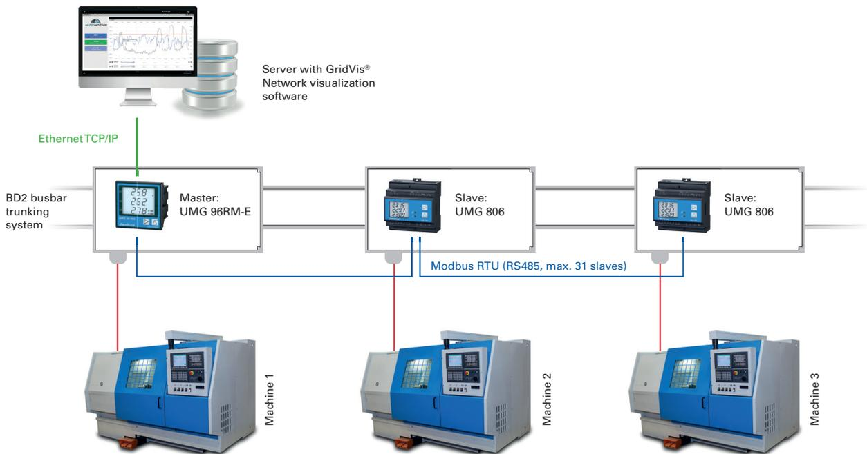
The busbar tap-off units (AKM) can be linked via Ethernet or RS485 and have an integrated Ethernet RS485 gateway. When the first AKM is connected directly to the Ethernet, as shown in the example, and the integrated gateway func-
