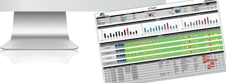
Keep track of system utilization\*: The report shows the utilization of all selected measurement points as a percentage and as an absolute value in the selected time period. Limit violations, excessive utilization, and reserves can be seen at a glance.
