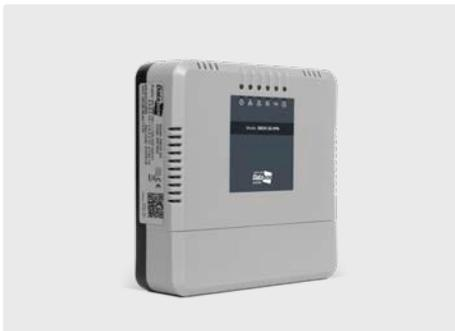
It's the brain of the installation. It is responsible for collecting data, generating alarms in real time, operating automatically and calculating KPIs.
