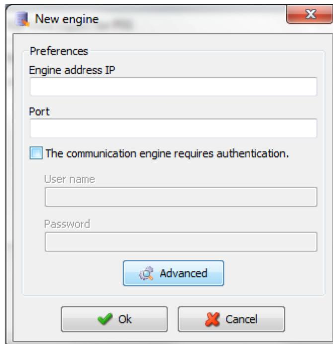
In this dialogue box, we can add the fields for the new engine such as the IP address and port. If the PSS engine has authentication activated, the username and password fields must be filled in for a valid user in this engine.
