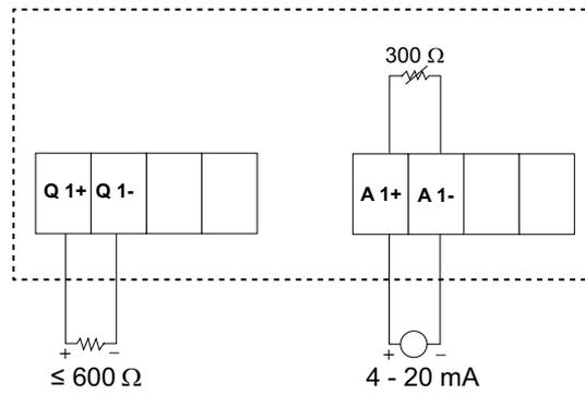
**Wiring the dual analog output**
