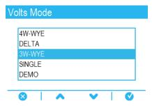
6. Press to confirm, and the new setting is applied to your meter. Press to cancel and maintain your meter's original setting.
