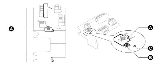
A Revenue lock switch coverB Sealing pointC Revenue LED
