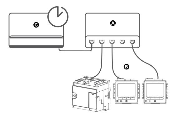
A Ethernet switch or hubB Ethernet connected metersC PTP master clock
