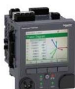
PowerLogic ION7400 with phasor display.
