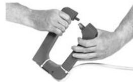
Twisting motion opens to CT diameter of round CT and smaller distance of rectangular CT.
