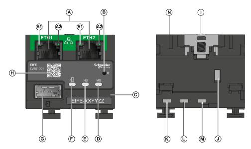
A Two RJ45 Ethernet ports
