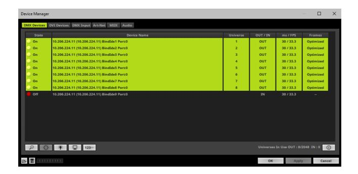
• [In the screenshot above, one LUNA 8 is connected. If more devices are connected, please use the different IP addresses of different devices and device details [i] to identify them in the Device Manager.]
