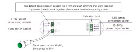
12V lamp connected, loads 0~144W(12V).
