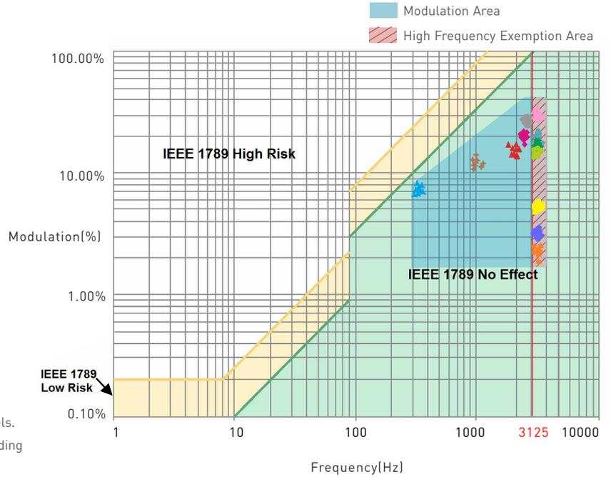
Marks in the right chart are tested results of different current levels. The output frequency is 0Hz in 100% brightness and its corresponding modulation is 0%, which could not be shown in the right chart.
