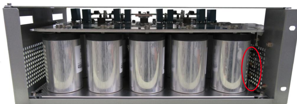
Figure 18: SEMiX5 stack back view with DC-link capacitors and discharge resistors
