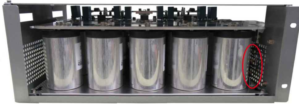
Figure 19: SEMiX5 stack back view with DC-link capacitors and discharge resistors
