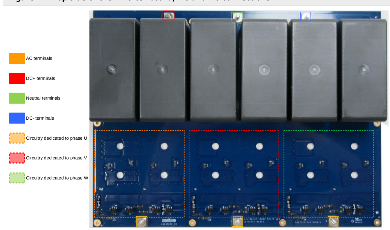
Figure 11: Top side of the inverter board; DC and AC connections
