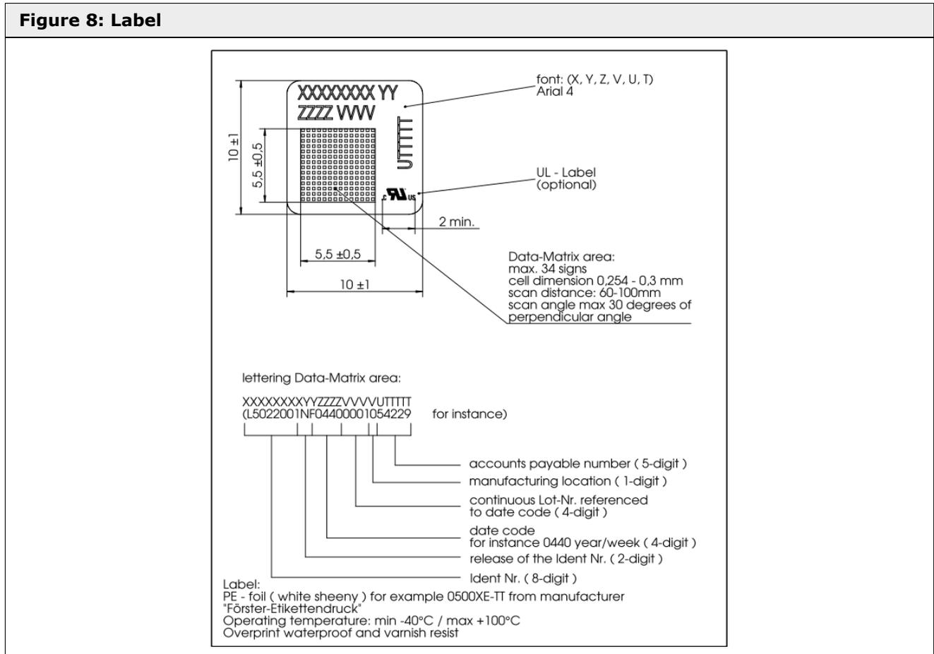
Every driver core is marked with a data matrix label. The marking contains the following items.
