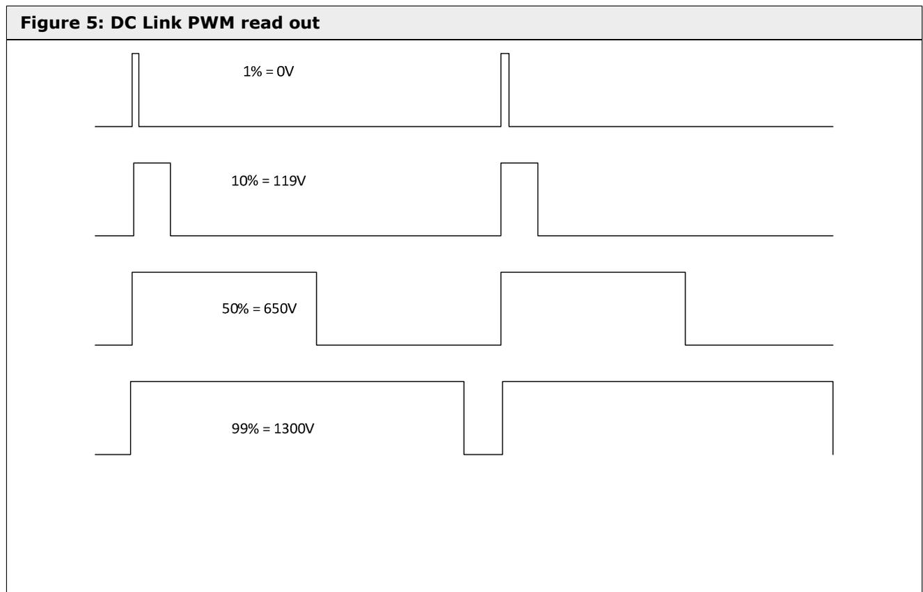
**Figure 6: Signal characteristic samples**
