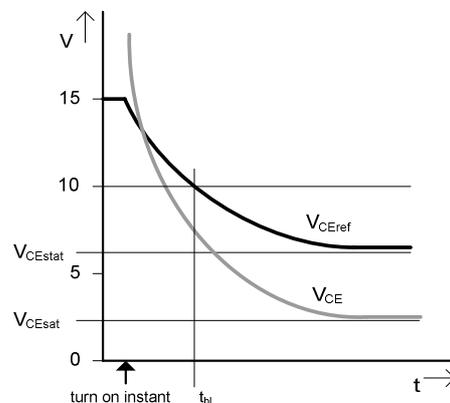
After  $t_{bi}$  has passed, the  $V_{CE}$  monitoring will be triggered as soon as  $V_{CE} > V_{CEref}$  and will turn off the IGBT. The  $V_{ce}$  monitoring settings is optimized to each module type and must not be adjusted by the user. The short circuit monitoring is set according to each module type separately. No further modification is necessary. Blanking time and threshold voltage is written in the datasheet.
