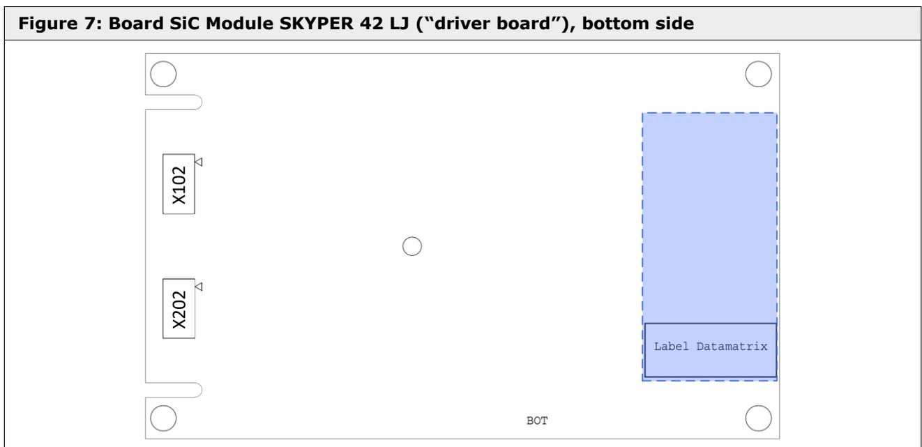
The plugs X102 and X202 (see Figure 7) on the bottom side contact directly to a SEMITRANS 3 module.
