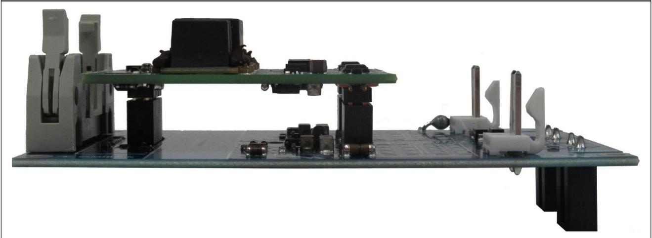
**Figure 4: Board SiC Module SKYPER 42 LJ**
