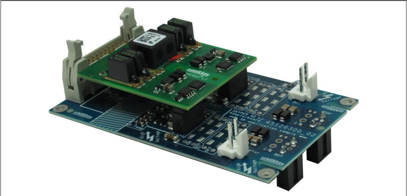
This Application Sample is dedicated to both universities and professional development engineers. It offers an easy way to bring 2L SiC MOSFET modules in operation. All Application Samples have been isolation tested; there is no functional routine test.
