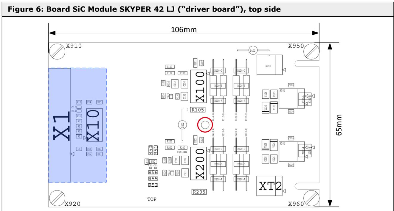
The blue marked area in Figure 6 and Figure 7 indicate the primary side with the user interface socket. The insulation is provided by the galvanic insulation of the SKYPER 42 LJ driver and the insulation gap on the driver board. All area besides the blue marking may be considered as high voltage area (secondary side).
