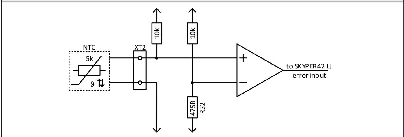
The standard value for R52 is 475Ω (refers to 100°C): the thermal overload detection is deactivated by not connecting the NTC-plug XT2 (framed brown in Figure 8).
