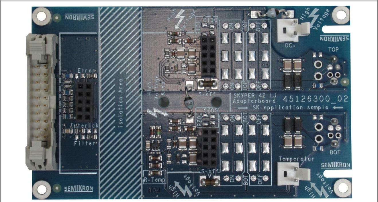
Depending on the power ratings and the operating conditions (voltage, current, and inductance of the DC-link connection) it might be necessary to adjust gate resistors, clamping voltage and trip levels of the safety circuits.
