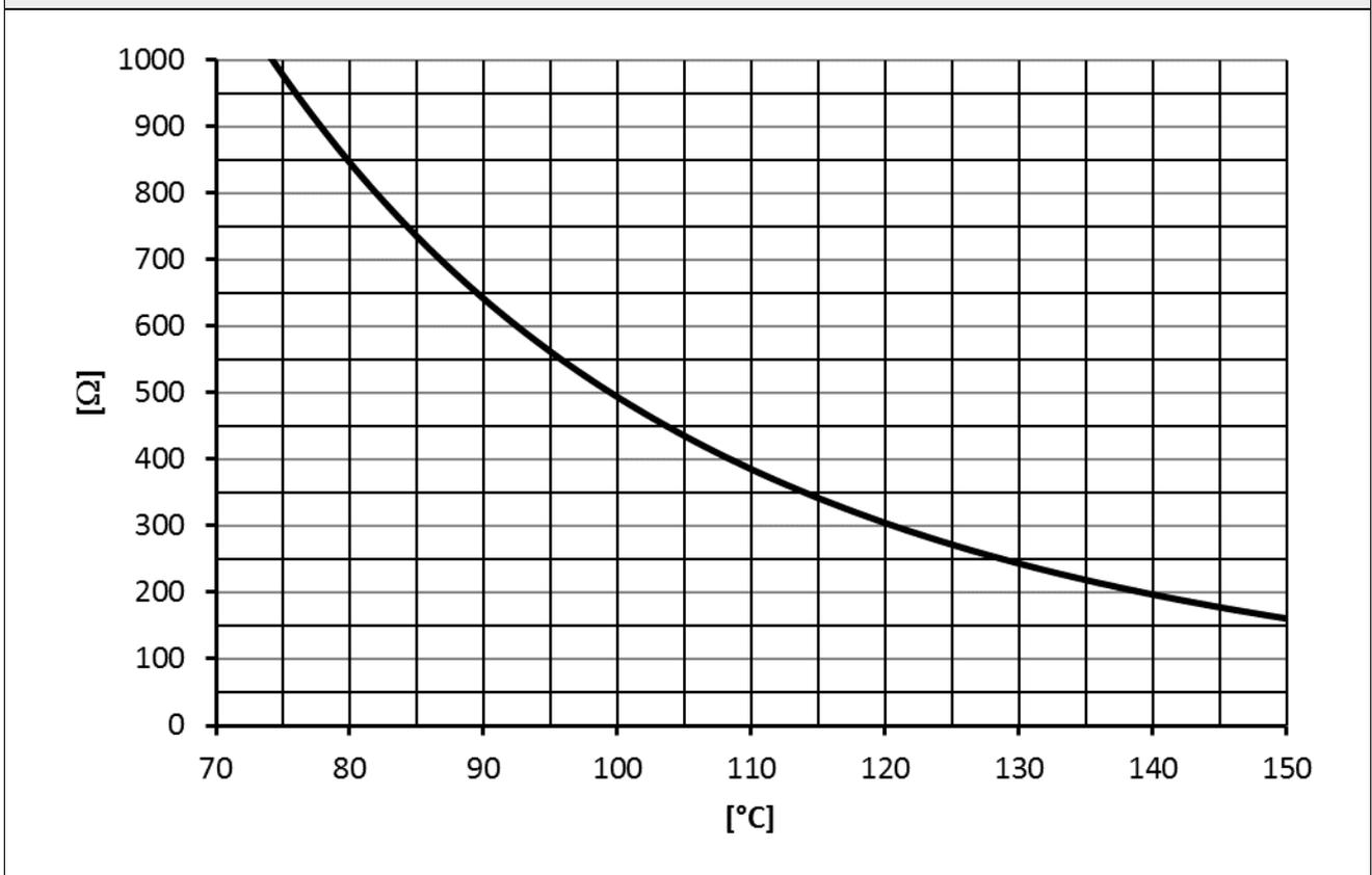
Figure 10 shows an excerpt of the SEMIKRON standard modules' NTC characteristic, which includes the most interesting temperature range between 70°C and 150°C. The full characteristic can be found in the Technical Explanation of the used module's datasheet or can be calculated from the formula given in the particular datasheets [1].
