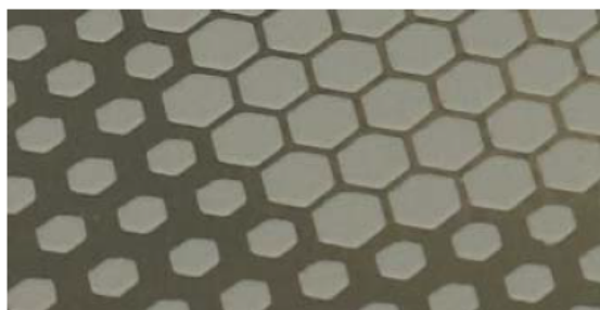
Figure 12: Application of PCM phase change material on SEMITRANS®10 baseplate and inhomogeneous honeycomb structure
