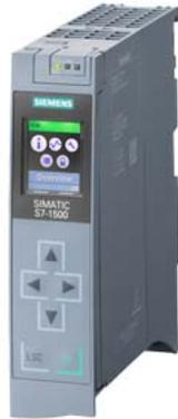
\*\*\* Spare part \*\*\* SIMATIC S7-1500, CPU 1513-1 PN, central processing unit with work memory 300 KB for program and 1.5 MB for data, 1st interface: PROFINET IRT with 2-port switch, 40 ns bit performance, SIMATIC Memory Card required
