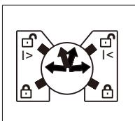
As shown in the figure above, they are wrong settings. In that cases , LED-U and LED-R will flash at the same time, which indicate the setting error. Normal operation will be resumed through resetting after power-off.
