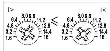
The set over-current threshold value must be larger than under-current threshold value. Otherwise, the two LEDs would flash and the output relay would be disconnected.
