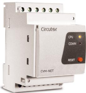
**CVM-NET-MC** is an instrument that measures and calculates the primary electric parameters in three-phase industrial power grids (balanced or unbalanced). It is measured in true RMS values, using three AC voltage inputs, and three AC current inputs (through current transformers  $I_h / 250\text{mA}$ ).
