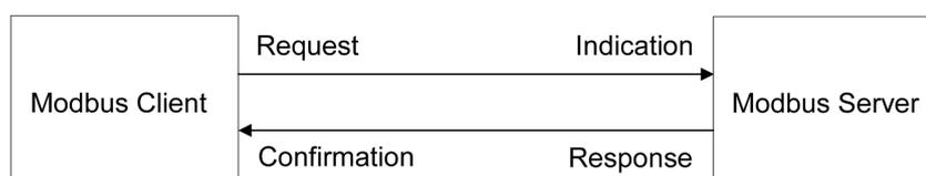
The Modbus messaging service implements client-server communication between devices connected by means of a TCP/IP network. Modbus TCP does not use an object dictionary.
