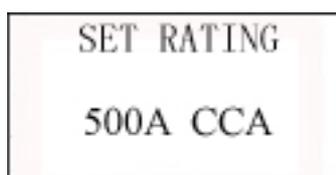
Input correct test standard and rating, press OK key, tester starts to test, and dynamic interface "TESTING" prompted. See below.
