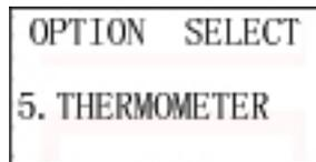
Press OK key to display the thermometer interface.
