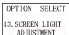
This function is to adjust the screen backlight brightness for power saving mode and for clear view of the displayed characters under the sunlight.
