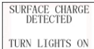
Turn lights on as prompted to eliminate battery surface charge, tester will then display the following messages in a sequence:
