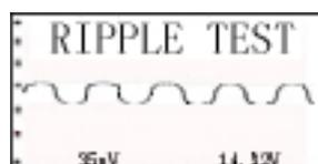
For ripple test, tester will display the real time ripple and meanwhile, shows ripple volt and charging volt values at the bottom line.
