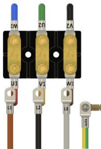
Low Voltage Delta Connection
