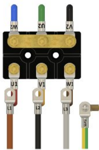
High Voltage WYE / STAR Connection
