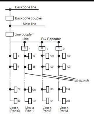
Fig.1. Connection of repeaters to a bus line
