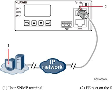
Figure 4-10 Connecting a communications cable (over SNMP)
