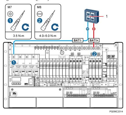
Figure 4-15 Installing battery cables for subrack
