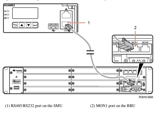
Figure 4-9 Connecting a communications cable (over the RS485 port)
