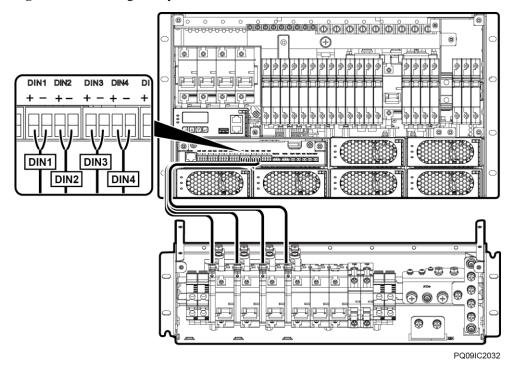
Figure 4-17 Installing battery circuit breaker detection cables for the DCDB
