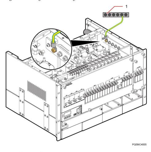
Figure 4-5 Installing the subrack RTN+ ground cable
