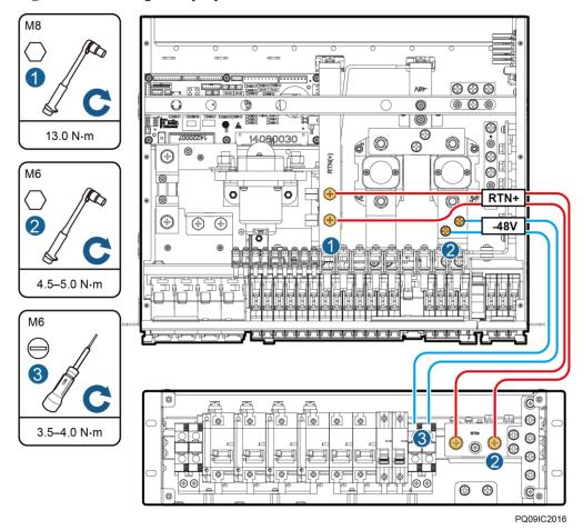
Figure 4-18 Installing DC input power cables for DCDB
