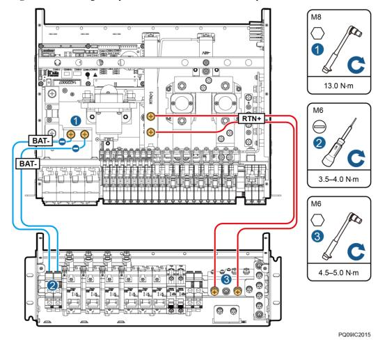
Figure 4-19 Installing battery cables between the DCDB and the power subrack
