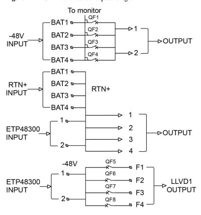
Figure B-2 DCDB electrical conceptual diagram
