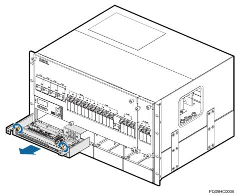
**Step 5** Record the positions where the UIM02C backplane connects to all the cables, and then disconnect the cables.
