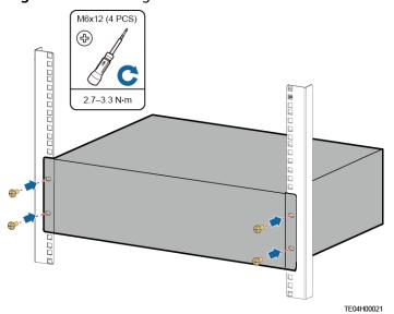
Figure 4-4 Installing the ETP48400-C3B1 or ETP48400-C3B2 subrack
