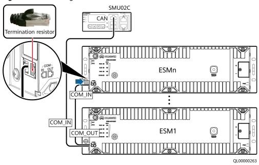
Figure 4-53 Installing communications cables for lithium batteries
