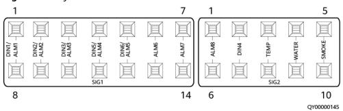
Figure 3-5 Pins in a COM port
