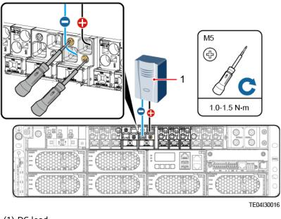
Figure 4-30 Installing DC output power cables
