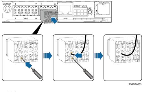
Figure 4-19 Installing a dry contact signal cable
