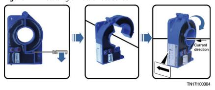
Figure A-2 Installing a Hall effect sensor 2
