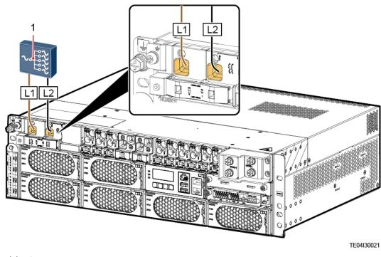
Figure 4-40 Installing AC input power cables
