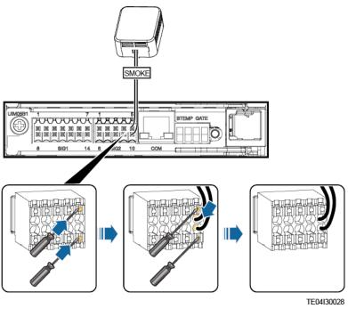
Figure 4-27 Installing smoke sensor cables
