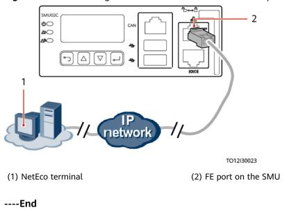
Figure 4-22 Connecting a communications cable to the FE port
