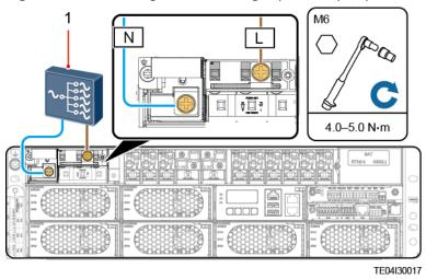
Figure 4-38 Installing 220 V AC single-phase input power cables
