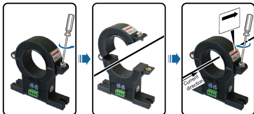
Figure A-2 Installing a Hall effect sensor 2
